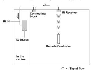
The IR IN input allows you to control the TX-DS898 from the remote zone (Zone 2) with the remote controller even though the remote zone is physically separated. The diagram below shows how to make the proper connections for the remote zone.
